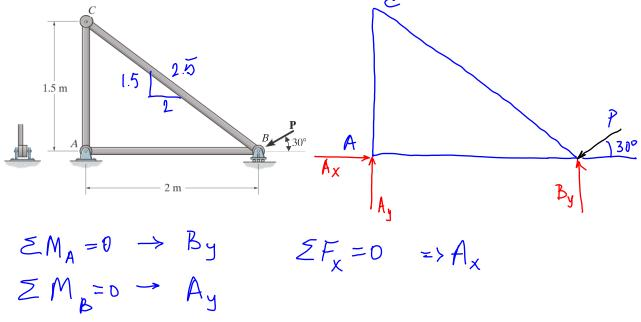
**Step 2** Draw a FBD for all of the individual joints. The internal forces of the members are directed along the length of each member.
